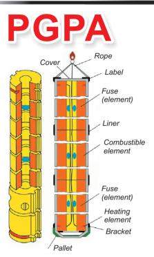
PGPA is the most powerful generator in Russia that has the largest weight of the charge. It increases the efficiency of well treatment due to the creation of high-frequency vibration during the firing of its elements that result in redistribution of the energy of the combusted products into the oscillatory component.
